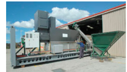
Figure 1: Torrefier being commissioned at AnthroTerra's workshops.
